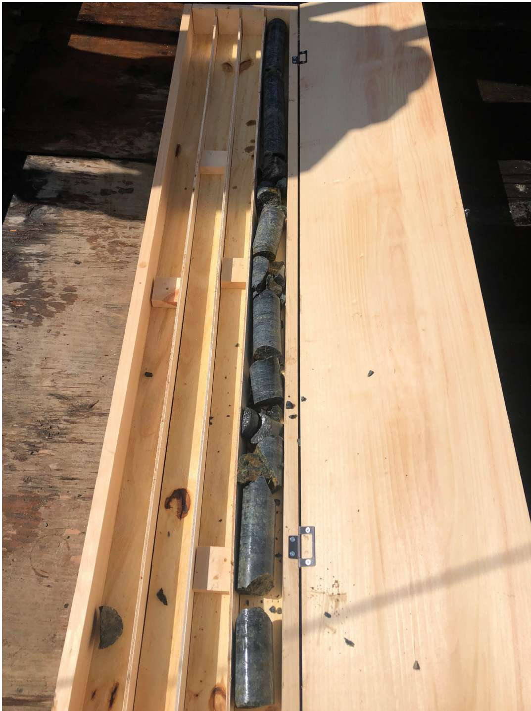
Figure C1: Boring B-2, C1 (75.5 – 80.5 ft) - Wet
