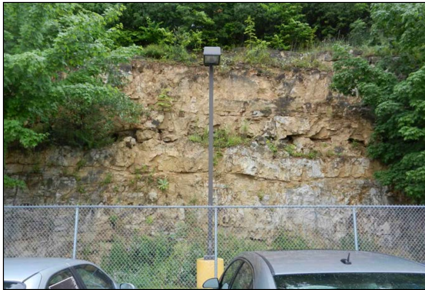
Figure 1: Photograph of rock exposure at Price Chopper parking lot northwest of the intersection of US2/US7 and Mountain View Drive. Solution cavity can be seen as horizontal zone about 1/3 of the way from the top of the exposure.
