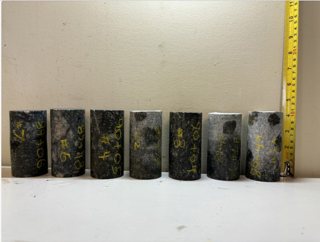
Rock core samples after saw cutting for compressive strength determination.
