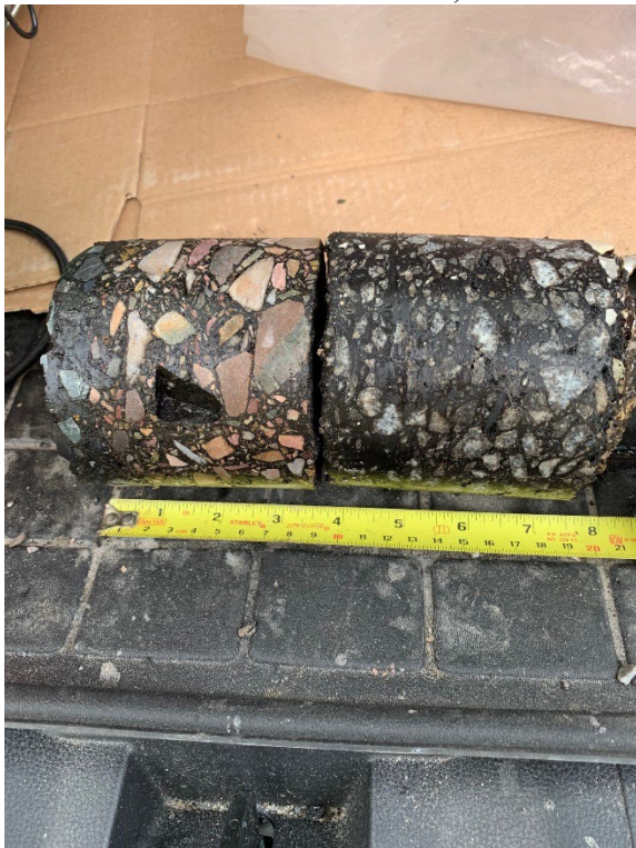
Asphalt core extracted at MM 55.0, Left Lane
