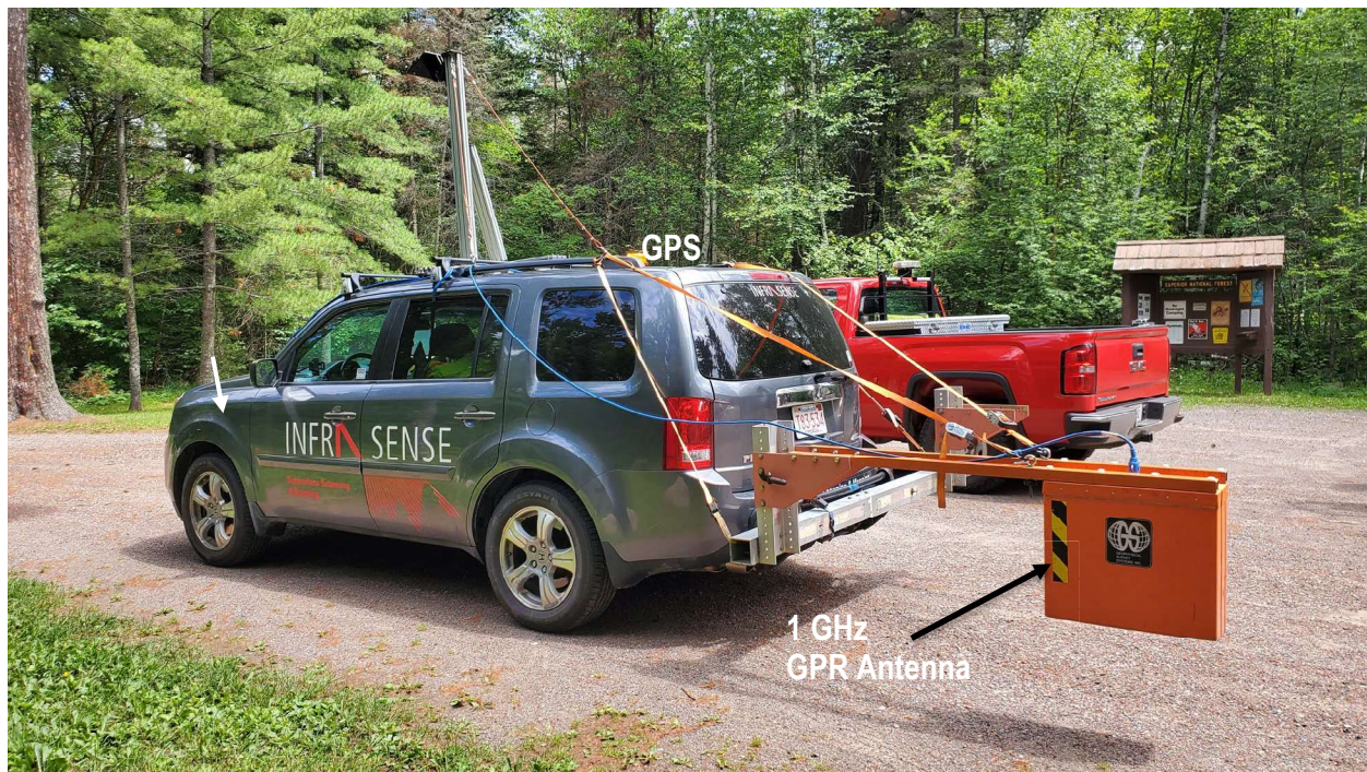
Figure 1 – Infrasense GPR Equipment Setup
