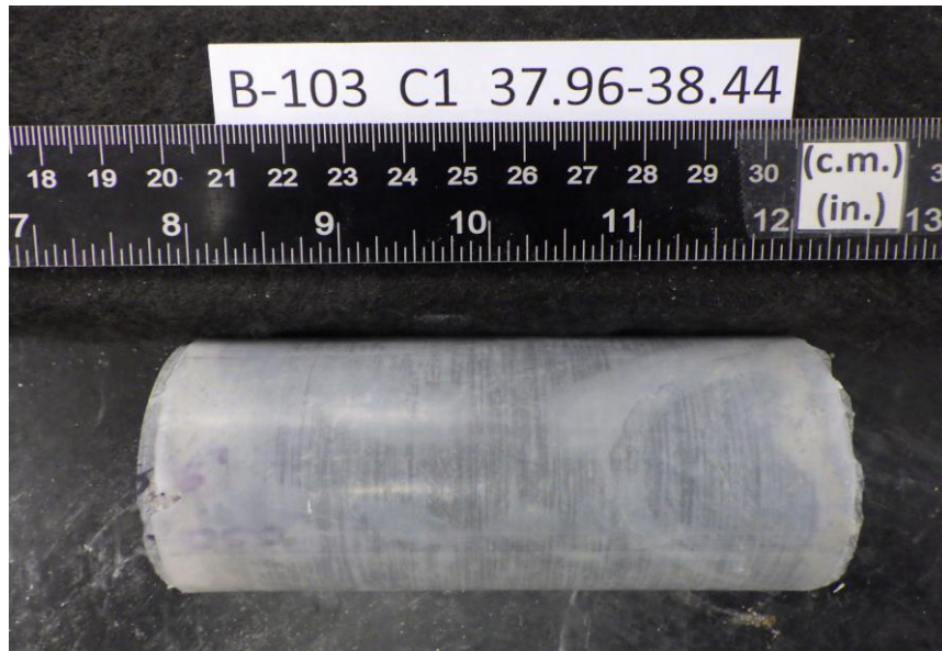
After cutting and grinding
