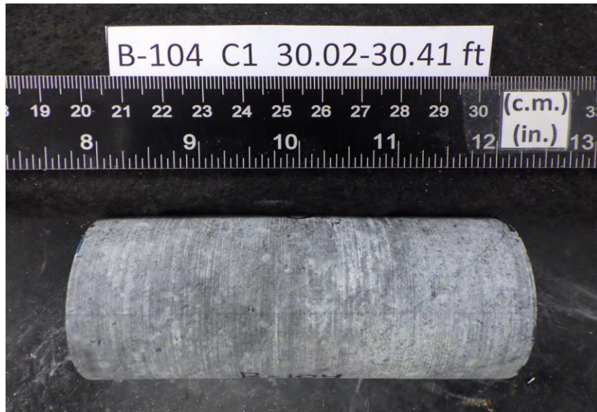
After cutting and grinding
