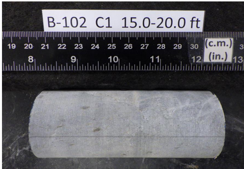
After cutting and grinding
