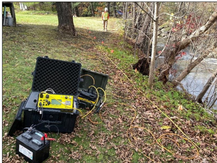
Figure 2-1: Setup of electrical resistivity imaging (ERI) system along ERI Line 2. Photo date November 5, 2021, view to the west.
