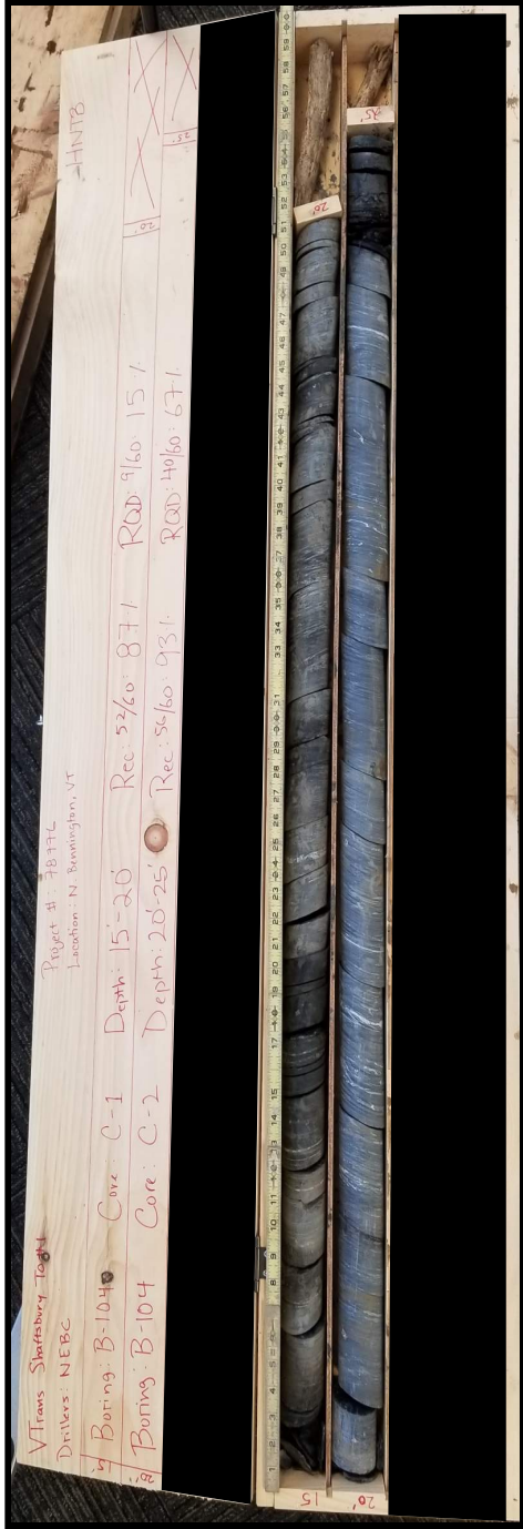
BORING B-104, ROCK CORES C-1 & C-2
